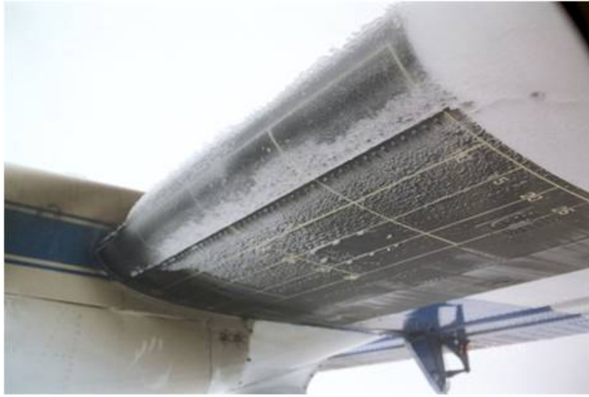
Figure 1.1 A typical ice accretion on an aircraft wing (courtesy: NASA Glenn Research Center).
